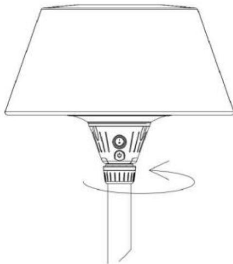
Step 6 : Fix the power cable with the pressure clips in the base.
