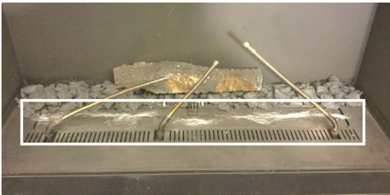
The "angel's hair" must be disentangled in length and deposit along the length of the burner according to the picture above.
